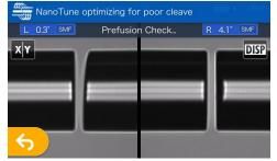
While splice program is selected to "AUTO NanoTune", the NanoTune™ analyzes the cleaved fiber surface and then sets up optimal splice condition.
