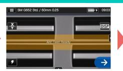
After "Arc Test Ready" appears, tap Set icon →. An arc test is started.
